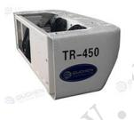
TR-450 model is front split mounted freezer unit, adopts R404a refrigerant, temperature is from  $-18^{\circ}$ C to  $+30^{\circ}$ C to deliver chilled or deep frozen cargoes. Its condenser and evaporator both have 2 fans respectively. It can apply for the medium refrigerated trucks or big pickup trucks.
